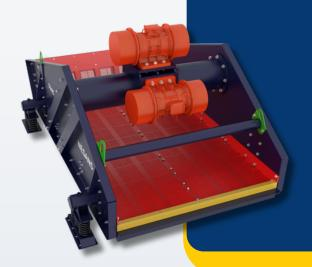
The Nesans D Series Dewatering Screens operate using high-frequency linear vibration to efficiently separate water from fine materials. Material is fed onto a steeply inclined screen deck where rapid vibration causes the particles to form a compact bed.
